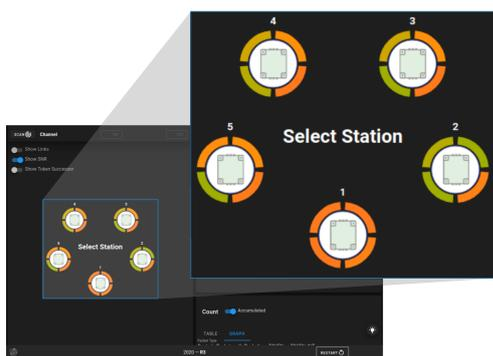
2. The topology now shows a graphical representation of the signal strengths between devices in network.
